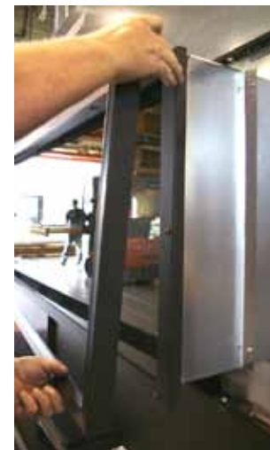
Figure 15. Step 2. (removal of Trim)
